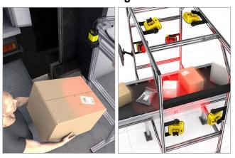
Overhead hands-free barcode reading stations or Modular Vision Tunnels decipher codes on various sides of a package, at extreme angles, and different orientations, reducing rework and lowering costs.
