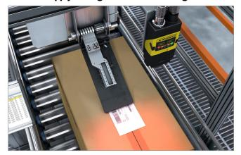
Cognex image-based barcode readers use code quality metrics and grading to identify and reject poorly printed codes attached during the inbound process, allowing facility managers to identify and fix printer errors to minimize problems downstream.
