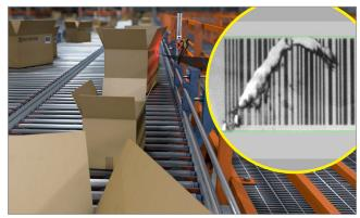
Image-based barcode readers catch label print and placement issues early on, allowing facility managers to identify and fix label or printer errors to minimize problems downstream.
