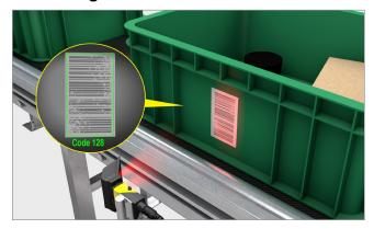
Image-based barcode readers, with advanced algorithms and decoding technology reliably read damaged, or non-aligned barcodes on totes in small egress situations to send them to the right pick station.
