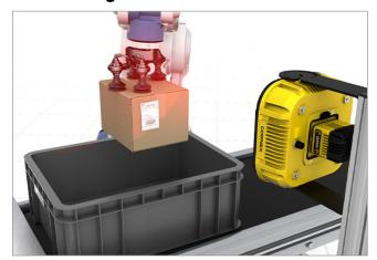
Reduce manual interventions and streamline efficiencies by scanning products and packages as they are transferred by a robot.
