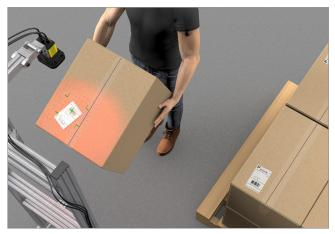
Deploying image-based barcode readers overhead helps facilities load outgoing trucks faster by enabling operators to build pallets more efficiently than using a hand scanner.
