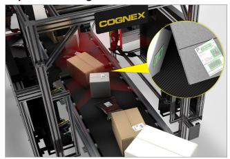
Cognex Modular Vision Tunnels are designed to read damaged codes at extreme perspectives on all sides of the box, even with the high speed and small gapping requirements of today's ship sorters. This allows a facility to increase throughput, without impacting sort accuracy.
