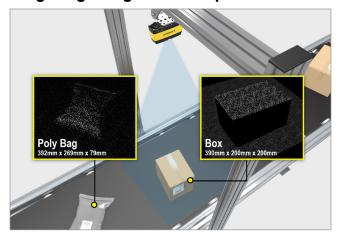
The 3D-A1000 Dimensioning System quickly and accurately categorizes products to ensure proper handling, which reduces damage to packages and keeps the sorter line moving smoothly.
