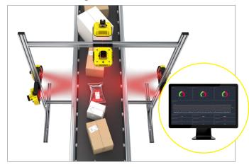
Modular Vision Tunnels help distribution centers improve accuracy and traceability of outbound shipping processes by providing a hands-free, efficient solution to verifying the correct packages are loaded onto the truck.
